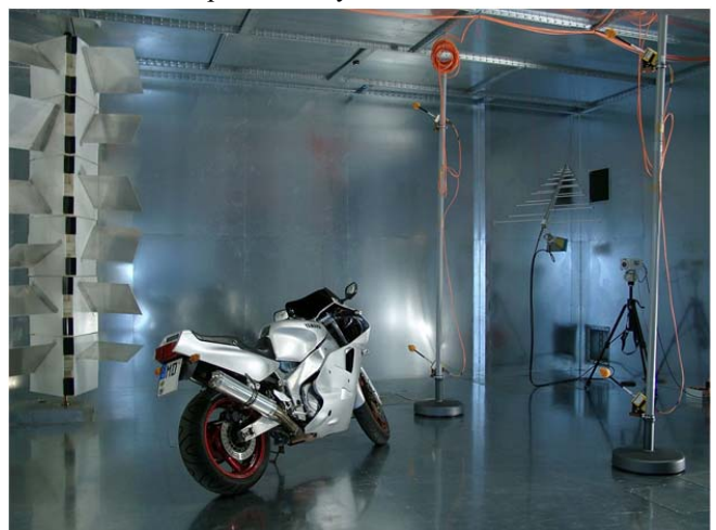
Figure 5: Example of a reverberation or stirred-mode chamber, the (large) Reverberation Chamber at Otto-von-Guericke-University Magdeburg, Germany
